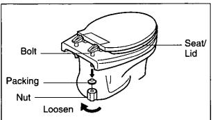
By using a wrench or other proper tool, release the nuts on both sides of the china bowl to remove the toilet seat and lid.
