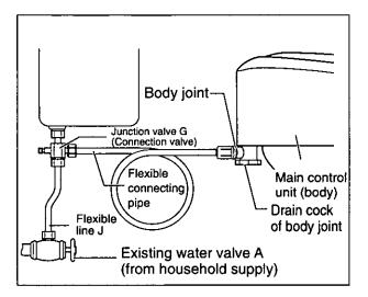
Connect the water branch outlet of the junction valve G to the body joint using the supplied flexible connecting pipe.
